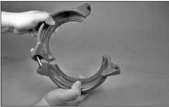
6. ASSEMBLE HOUSINGS: Insert one bolt into the housings, and thread the nut loosely onto the bolt to allow for the “swing-over” feature, as shown above. NOTE: The nut should be backed off no further than flush with the end of the bolt.
