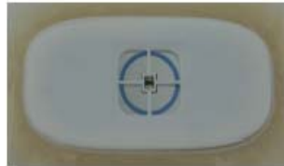
Fig. 5. The assembled patch with a pulse oximetry sensor made as a concentric photodiode around two LEDs placed in the center. The little square frame around the LEDs is to prevent light going directly from the LEDs into the photodiode.
