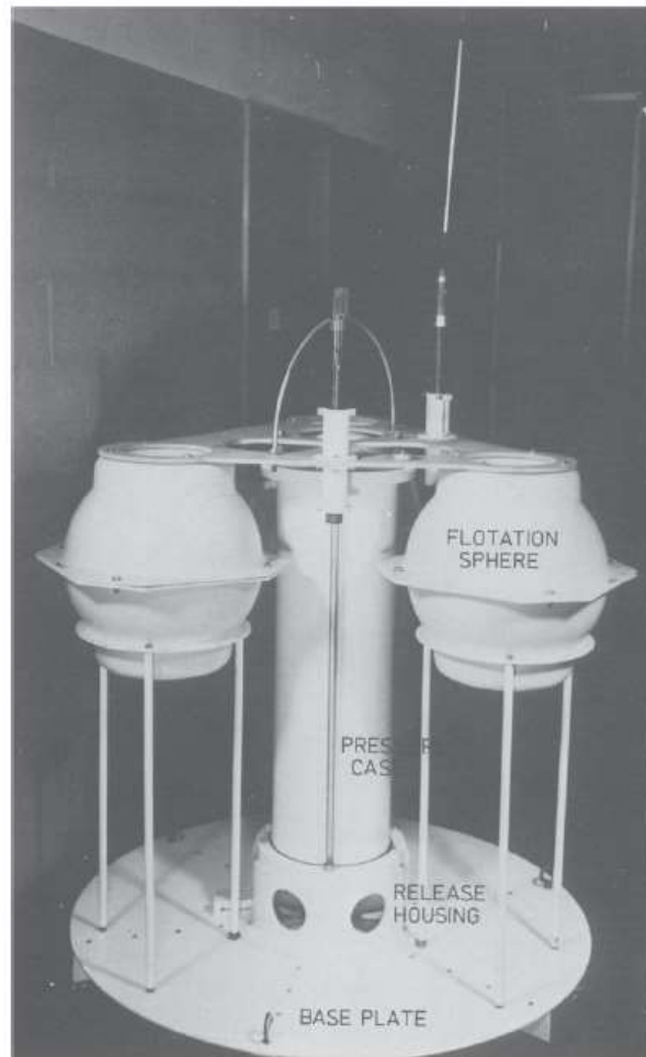
Fig. 1. MITOBS, external view. Visible are the pressure case, the flotation assembly and recovery aids, the lever arms and mechanical dogs of the release assembly, and the expendable base plate.
