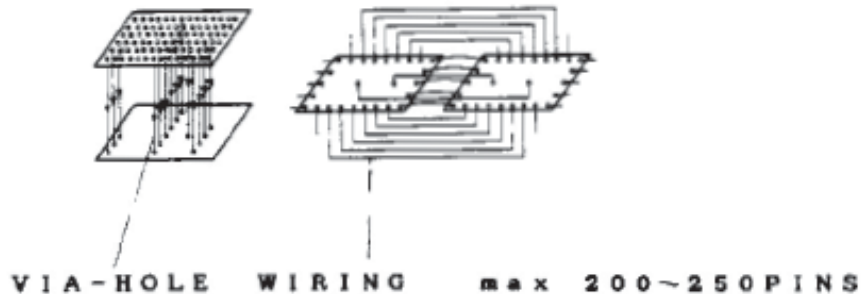
Fig. 4. Wiring for parallel processing in 2-D and 3-D ICs.
