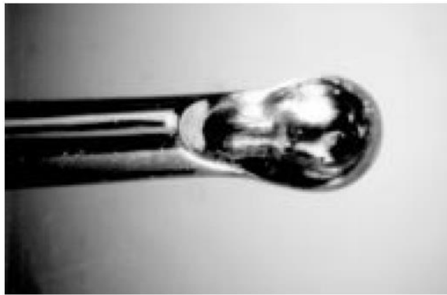
Figure 1 The tip of the ‘gonioscraper’. The bowl is 300 \mu m in diameter with its edges sharpened.
