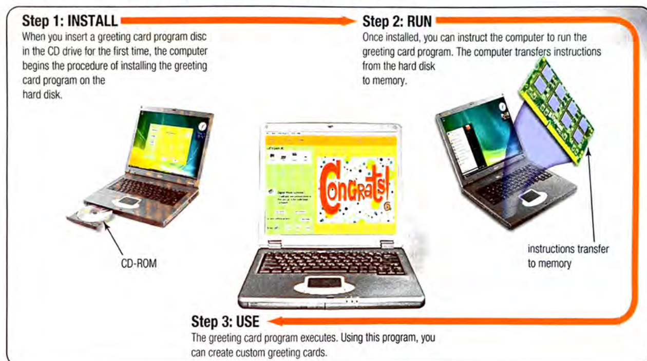
FIGURE 1-10 INSTALLING AND RUNNING A COMPUTER PROGRAM
