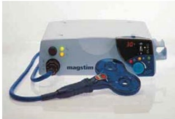
Figure 13 of Magstim, above, is a photograph of a Magstim 200 magnetic stimulator with a double coil. Id. at 9.
