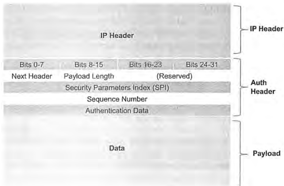
Figure 6.15: The authentication header.
