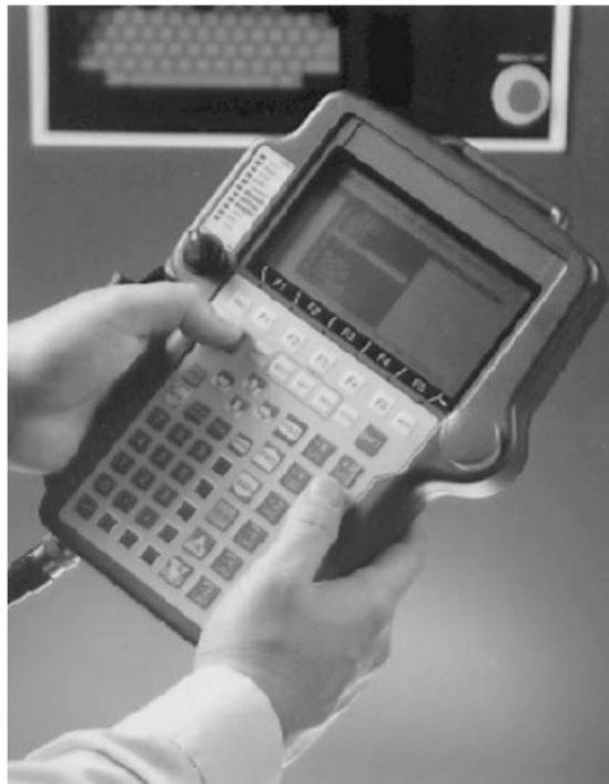
Figure 2 Teach pendant (courtesy Fanuc Ltd., Yamanashi, Japan).
