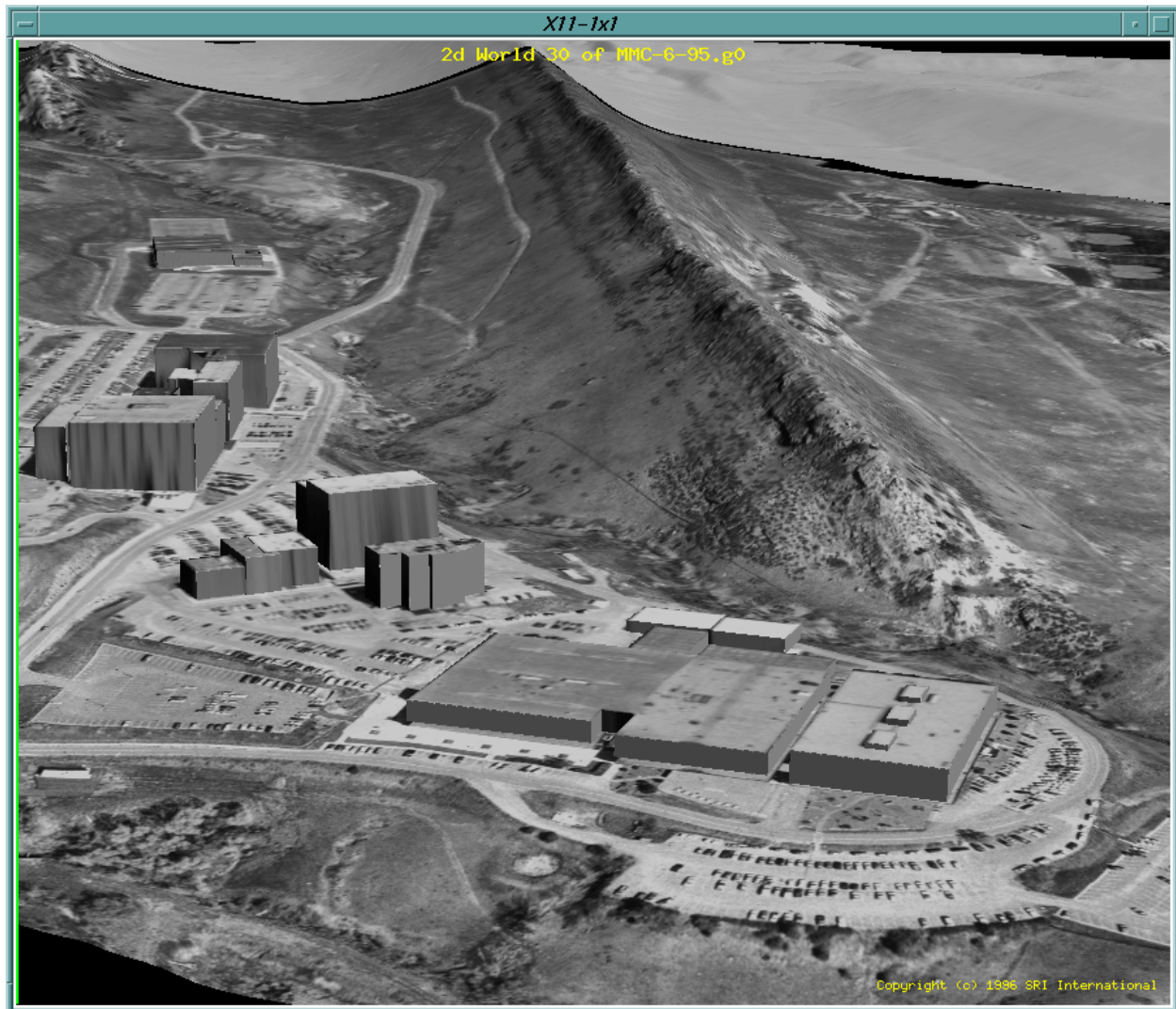
Figure 2: A synthetic view of a site constructed with the RCDE. The texture maps used on the models were automatically extracted from the appropriate images. The terrain model was created by F. Raye Norvelle of the U.S. Army Topographical Engineering Center using his Iterative Ortho-Refinement (IOR) technique.
