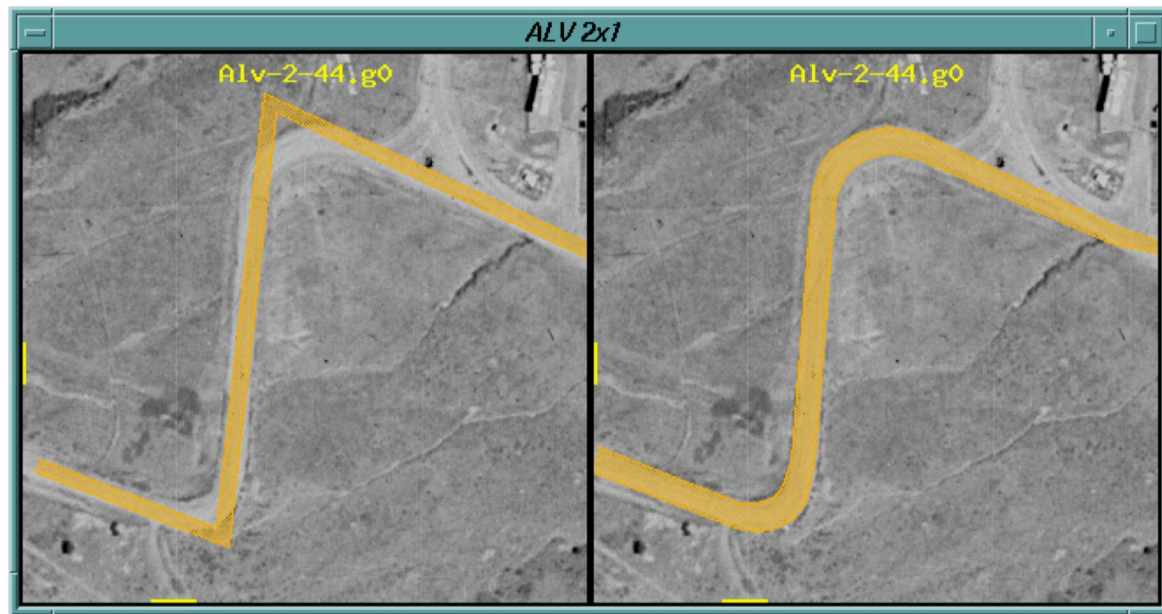
Figure 3: A road model, before and after optimization.
