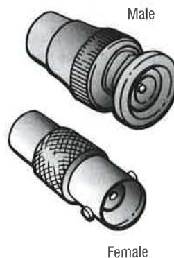
FIGURE 1.11 A male and female BNC connector
