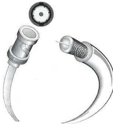
FIGURE 1.10 A stripped-back Thinnet
