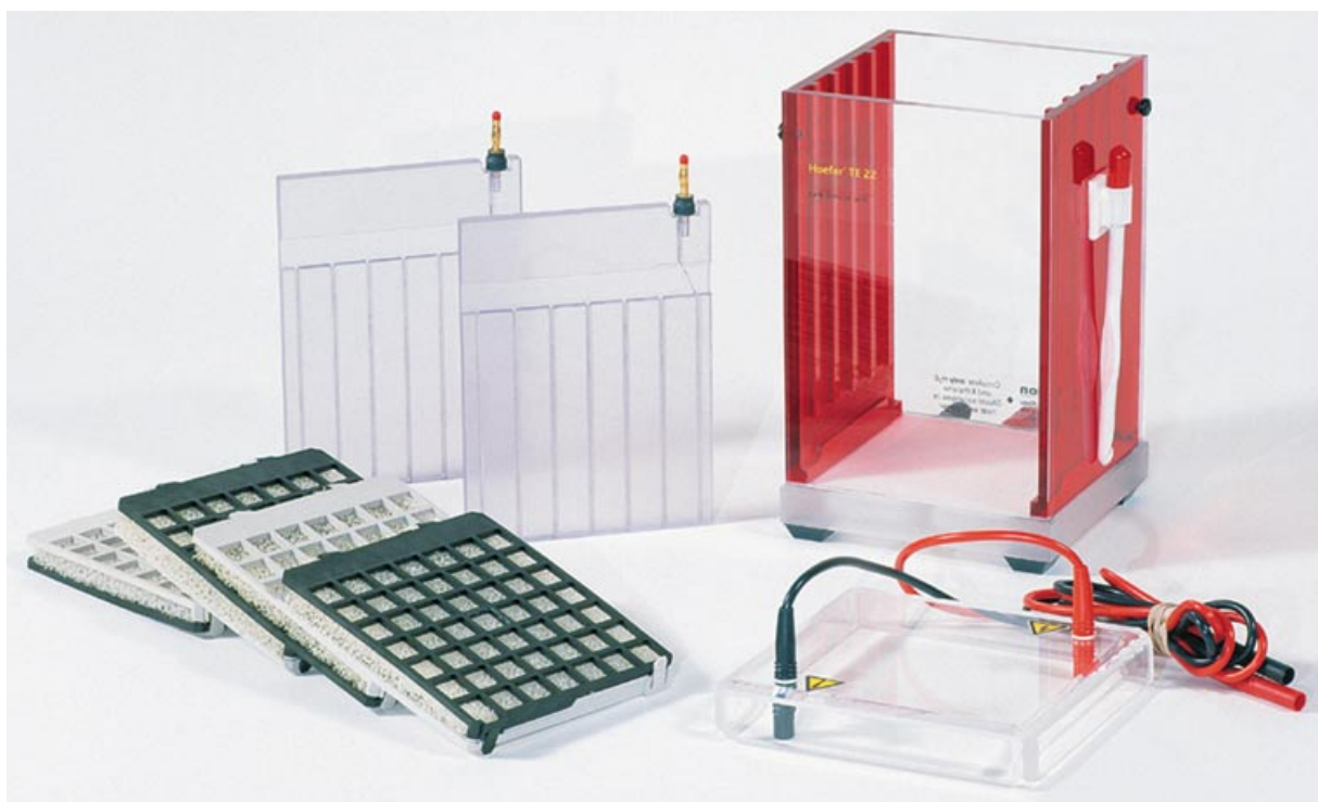
Figure 6.2.2 Minigel tank electrotransfer unit. Designed for smaller (8 × 10-cm) gels, these units will process four gels at a time. Note that the two outside panels hold the electrode grid.
