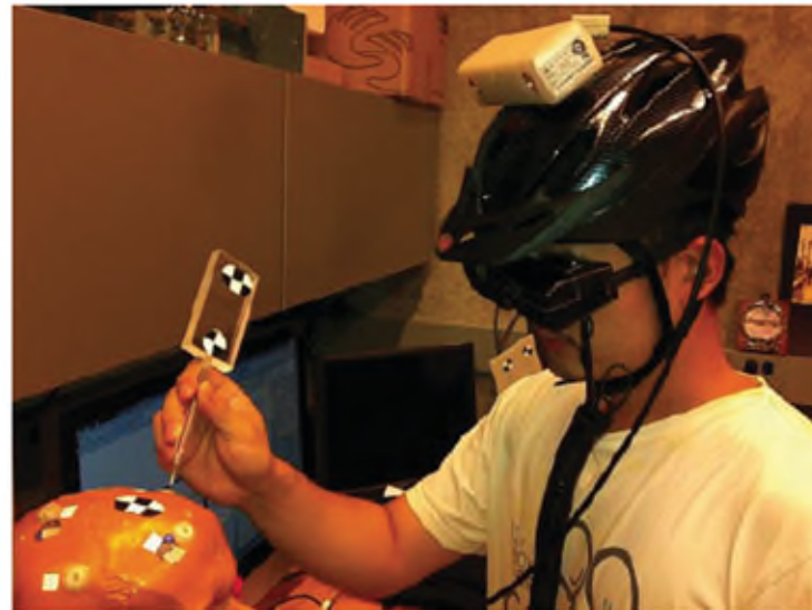
Figure 1. User wearing the optical see-through goggles and head mounted tracker. Figure shows the registration procedure, where the surgeon touches markers using a tracked probe.
