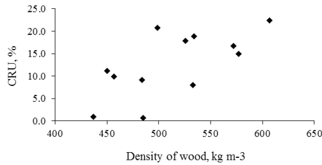
Figure 4. Relationship between relative increment of deflection and density of wood.
