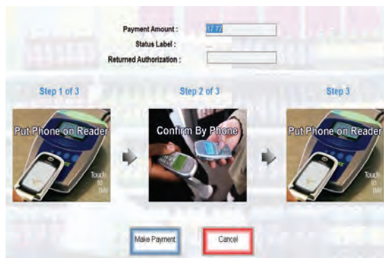
Figure 5. Mobile phone to local machine interaction (the left-hand side screenshot shows the steps displayed on the RSA based kiosk to guard user interaction, and the right-hand side screenshot shows payment confirmation on the mobile phone).
