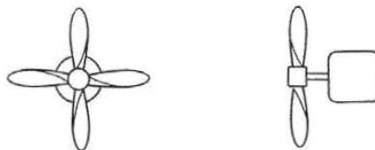
Figure 6.22 Typical small propeller fan.
