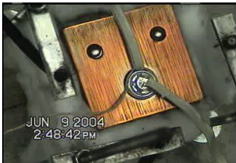
Figure 4. Thermal ramp apparatus with 18650 cell.
