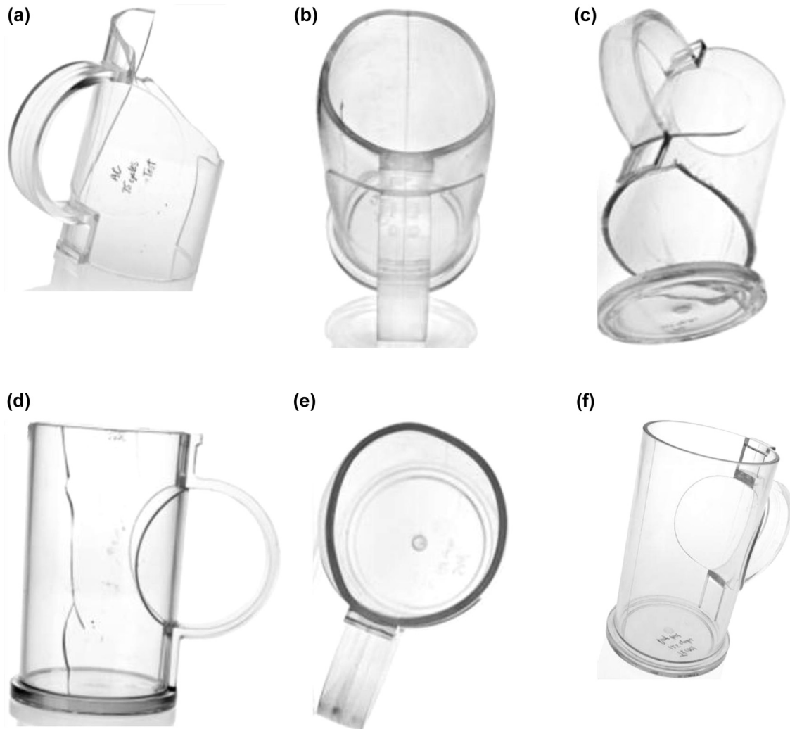
FIGURE 20.13 Photos of dishwashed mugs after respective number of residential dishwasher (DW) cycles, molded from (a) acrylic after 75 DW cycles and drop test, (b) methacrylate styrene after 50 DW cycles and drop test, (c) polycarbonate after 125 DW cycles and no drop test, (d) styrene acrylonitrile (SAN) after 30 DW cycles and drop test, (e) SAN after 125 DW cycles and no drop test, and (f) Tritan™ after 125 DW cycles and drop test. Photographs provided by courtesy of Eastman Chemical Company.
