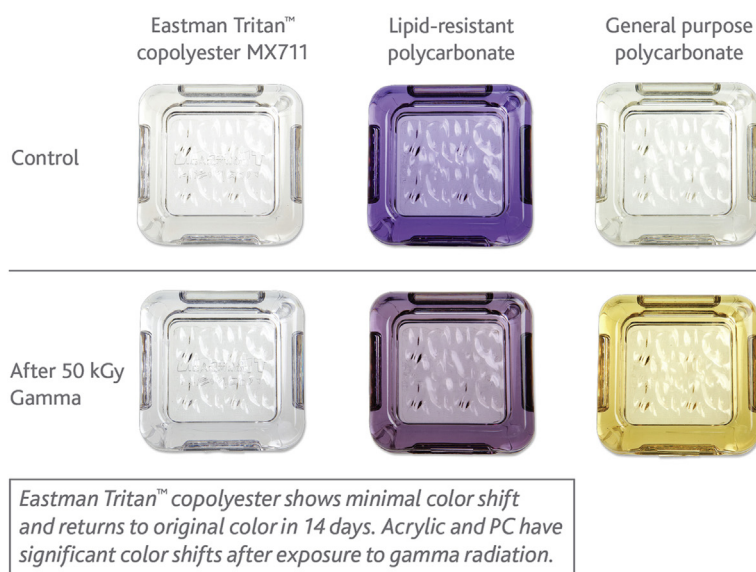
FIGURE 20.14 Color shift measured using CIELAB color ( b^* ) and visual color assessment of Tritan™ MX711, gamma-resistant polycarbonate (PC) and standard grade PC and acrylic after 50 kGy of e-beam radiation. Positive and negative b^* values correspond to a yellow (light gray in print versions) and blue (gray in print versions) hue, respectively. Photographs provided by courtesy of Eastman Chemical Company.
