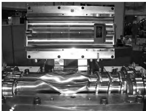
Figure 4.9 Farrel continuous mixer. Courtesy: Farrel Corporation
