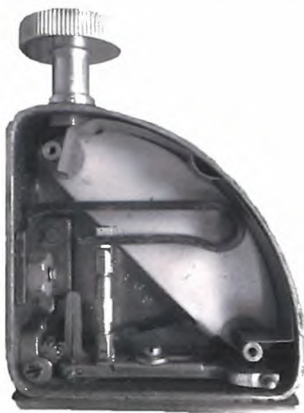
FIG. 1—Shore quadrant scale D durometer.
