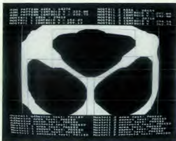
Fig. 4. Structural adhesive pattern image after processing and analysis, showing test data and results.
