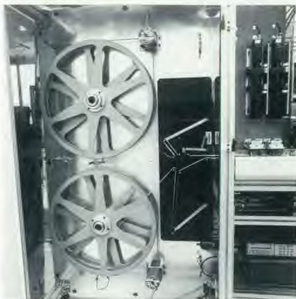
Fig. 6. A view of the automatic print quality tester showing the paper feed and take-up reels and tension arms.
