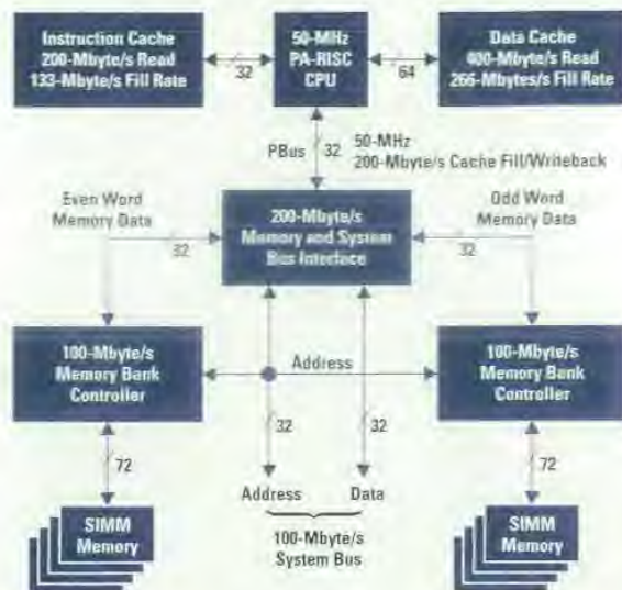
Fig. 3. Memory and system bus interface interconnect ports.
