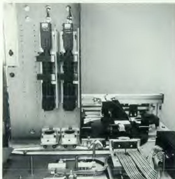
Fig. 5. A view of the automatic print quality tester showing the illuminators, cameras, optics, rotary table, and print cartridge nests.
