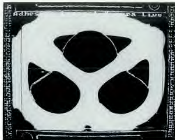
Fig. 3. Unprocessed image of the structural adhesive pattern.
