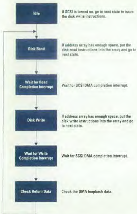
Fig. 4. Operation of the bus exerciser's SCSI state machine.
