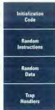
Fig. 3. Structure of a BPS test.
