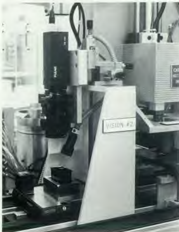
Fig. 1. The filter stake inspection station uses off-axis illumination and polarizing optics.
