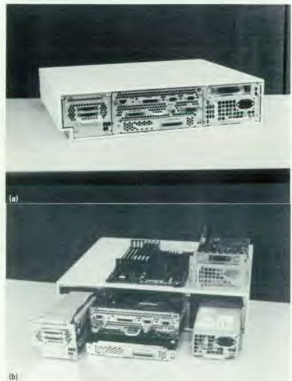
Fig. 2. Access to the disk tray, CPU board, I/O board, graphics board, EISA board assembly, and power supply is from the rear.
