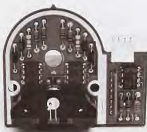
Fig. 5. An encoder previously used in many HP plotters. It had 28 parts. The HEDS-9000 module that replaced it has five.
