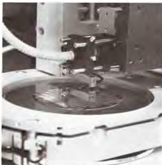
Fig. 3. Inkjet printheads being removed from the low-tack mounting tape in the head attach machine.
