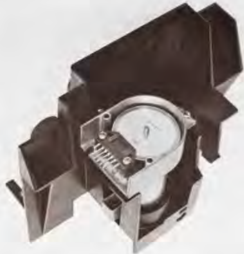
Fig. 1. The HEDS-9000 encoder with code wheel mounted on the DeskJet printer carriage drive motor.
