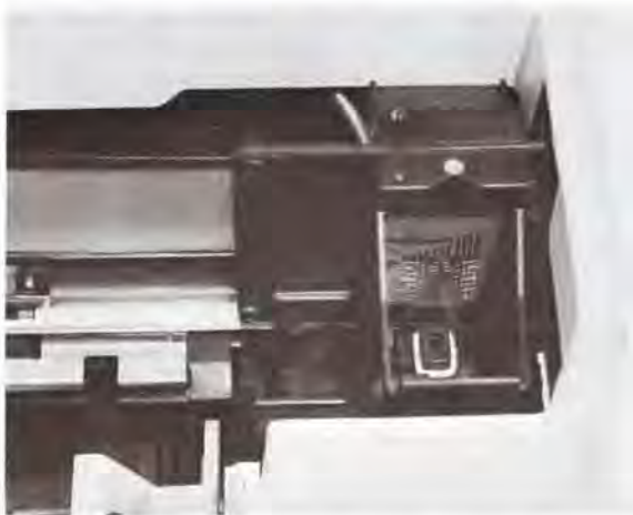
Fig. 2. For interconnecting the printer and the printhead, the DeskJet printer uses a bumped flex circuit on the carriage.
