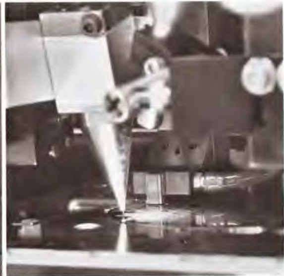
Fig. 2. An orifice plate being optically aligned to a whole wafer in the orifice attach machine.
