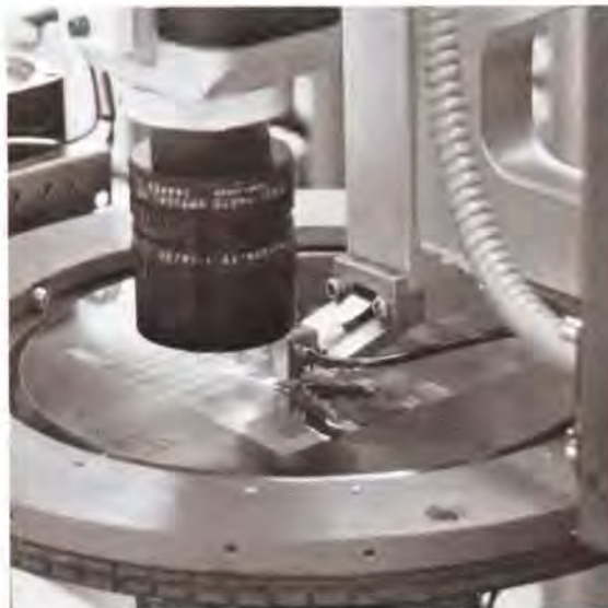
Fig. 1. Orifice plates being removed from the low-tack mounting tape in the orifice attach machine.
