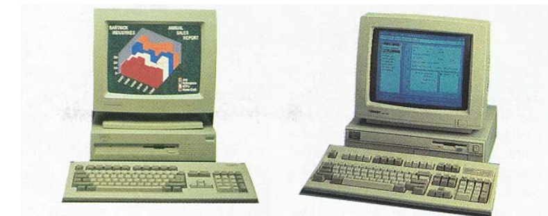
FIGURE 6a-b. New Multimedia Computers from Commodore and Tandy. Like the Macintosh, the Commodore Amiga 3000 uses the Motorola 68030 CPU, but the price is much lower than Apple's. Earlier Amigas have done well in television and music applications, and with the 3000, Commodore hopes to crack the business and education markets. The Tandy 2500 XL meets Bill Gates' specification for a low-end multimedia machine. It is an AT-compatible PC with a CD-ROM drive audio processing chip.
