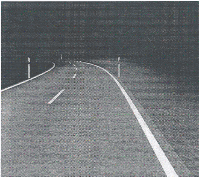
Fig. 9: Conventional luminous intensity distribution
