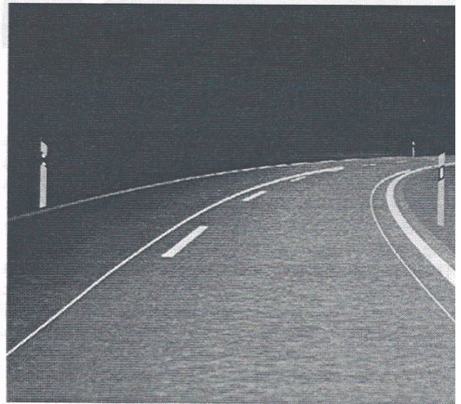
Fig. 8: Control of the headlamps with path prediction
