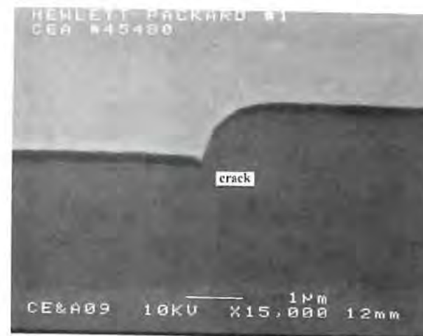
Figure 5.8 Ni-Au bump with a crack in the passivation.
