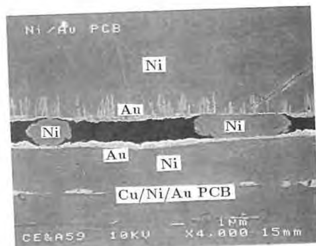
Figure 5.21 ACF bonded flip chip with Ni-Au bump on Cu Ni Au PCB.
