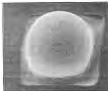
Figure 2.70 Twice-reflowed Tacky Dots solder bump.
