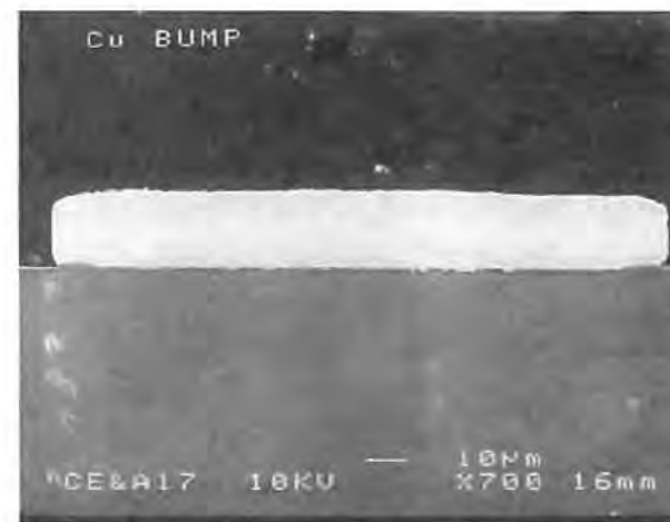
Figure 5.5 A typical Si chip with Cu bump.
