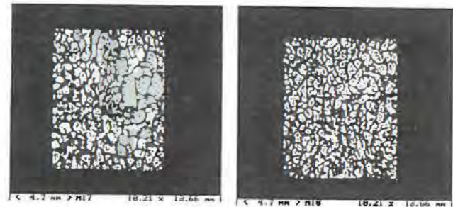
Figure 5.26 C-mode images of die bonded on the original PCB (left) and prebaked PCB (right) with adhesive A.
