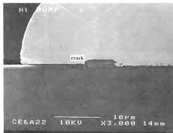
Figure 5.7 Ni-Au bump with a crack in the passivation.
