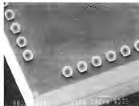
Figure 2.60 Micro solder bumps with 140- \mu\text{m} pitch (initial ball diameter: 80 \mu\text{m} ; number of bumps: 200).
