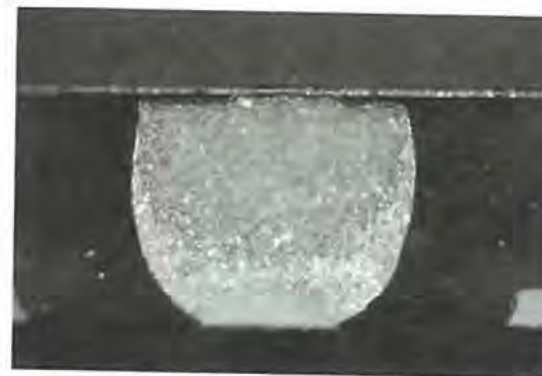
Figure 6.5 Cross section of IBM's low cost FCOB.
