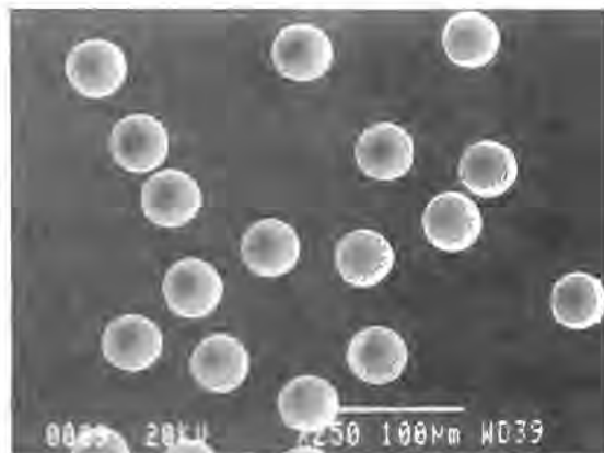
Figure 2.54 SEM image of micro gold balls (45 \mu\text{m} in diameter).
