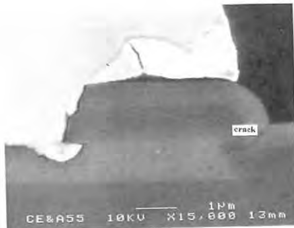
Figure 5.11 Ni Au bump with a crack in the passivation.
