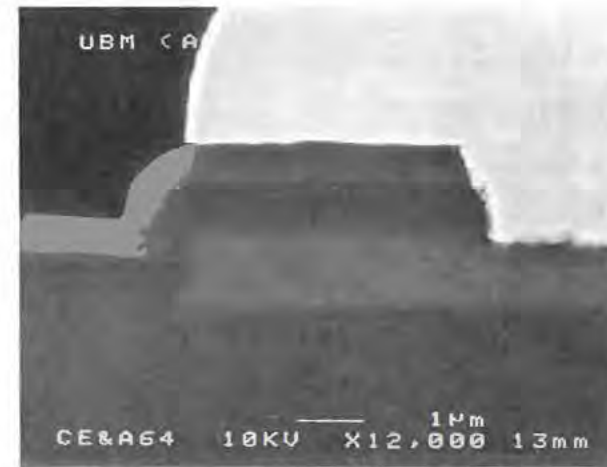
Figure 5.12 Ni Au bump with no cracks (a perfect one!).
