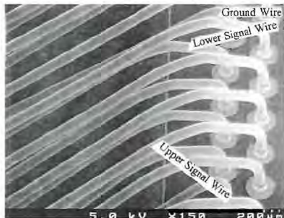
Figure 2.4 Magnified SEM image of the bonding wires at the chip area.
