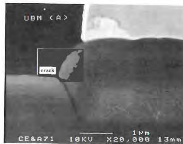
Figure 5.9 Ni Au bump with a crack in the passivation.
