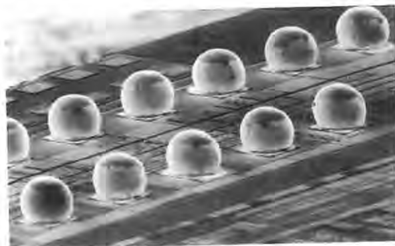
Figure 2.8 SEM photograph of solder bumps on chip.
