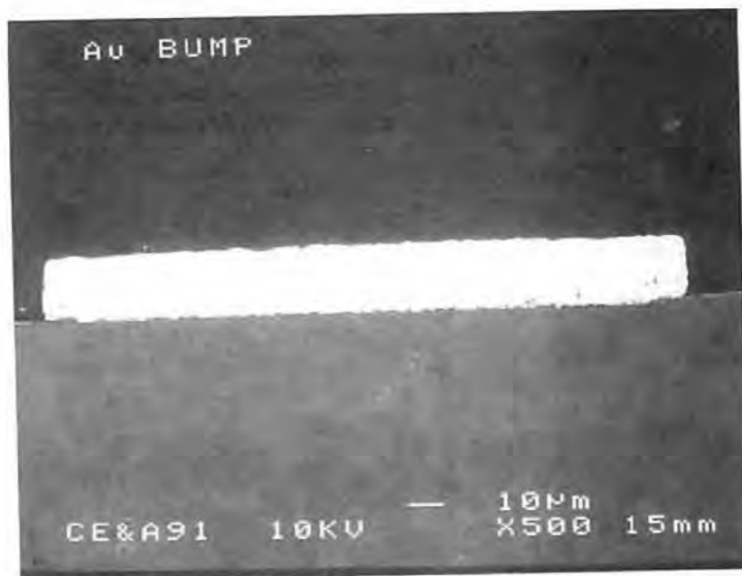
Figure 5.4 A typical Si chip with Au bump.
