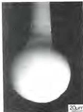
Figure 2.74 SEM photo of the solder alloy ball formed by arc discharge.
