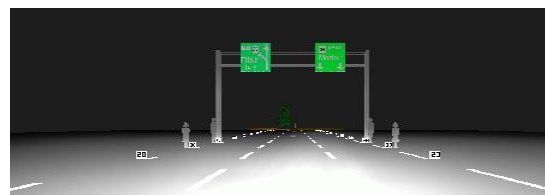
Fig.11B The road render of test results of the LED low beam head lamp
