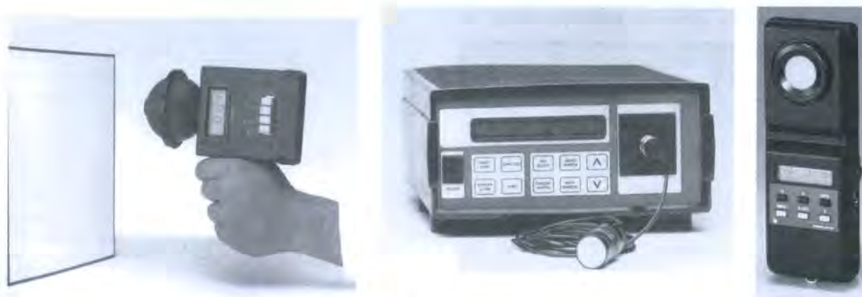
Figure 2-7. Various commercial illuminance meters. (a) Portable illuminance meter with small integrating sphere; (b) laboratory grade system that includes a photometer, a radiometer, and a fiber-optic power meter; (c) multifunction portable illuminance meter with detachable receptor head.
