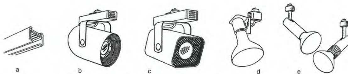
Figure 7-19. Examples of track luminaires: (a) close-up of multicircuit track, (b) and (c) track-mounted luminaires with optical control, and (d) and (e) track luminaires for holding and aiming lamps.
