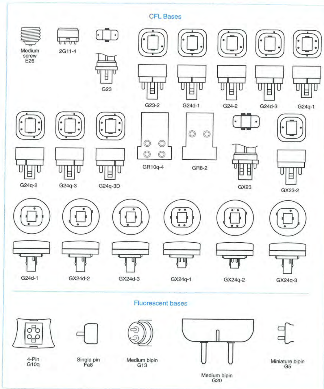
Figure 6-29. Typical bases for linear and compact fluorescent lamps (not to scale). ANSI designations are shown.
