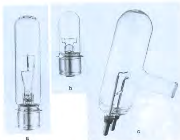
Figure 6-23. Typical ribbon filament lamps: (a) 6-volt, 18-ampere, T-10, 2-mm, 3000-K microscope illuminator; (b) 6-volt, 9-ampere, T-8½, 1-mm, 3000-K optical source; and (c) 3.5-volt, 30-ampere, T-24 with quartz window, 3-mm, U-shaped filament, 2300-K pyrometer and spectroscopy source.
