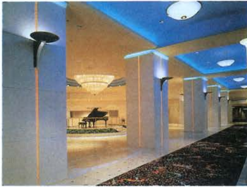
Plate 5. A festive, yet elegant mood was created for an entrance to a hotel and casino. The main lighting features include strings of low-wattage incandescent lights inserted into column slots, translucent alabaster column capitals that conceal fluorescent striplights, halogen wall sconces, blue neon cove uplight, incandescent bowl pendants, and PAR38 halogen downlights.
