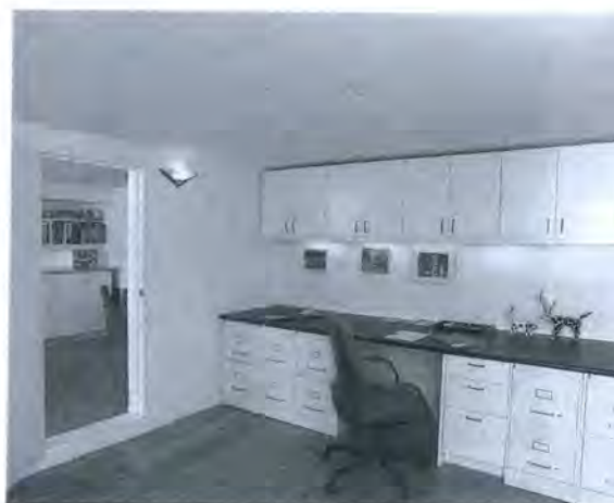
Figure 18-3. A home office is illuminated with several types of lighting: recessed downlights for general lighting, under-cabinet luminaires for task lighting on the desk top, and a wall sconce for style.
