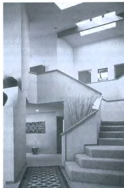
Figure 18-5. Left, a three-dimensional effect was created for the lighting of this hallway. Three recessed PAR-30 spotlights were used to wash the wall of the upper hallway and give depth to the view. The open passageway was lighted with wall-mounted up/down fluorescent lamp luminaires. A low voltage incandescent strip was used to light the railing. The bottom step of the staircase was illuminated with a downlight, while the dried reeds were illuminated with uplight. This lighting scheme plays with various brightnesses and emphasizes three-dimensional planes and depths. Right, a daytime view of the same hallway. While the skylight is pronounced, the three-dimensional features of the lighting scheme are not as noticeable.
