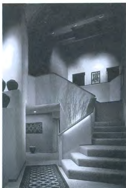
Figure 18-5. Left, a three-dimensional effect was created for the lighting of this hallway. Three recessed PAR-30 spotlights were used to wash the wall of the upper hallway and give depth to the view. The open passageway was lighted with wall-mounted up/down fluorescent lamp luminaires. A low voltage incandescent strip was used to light the railing. The bottom step of the staircase was illuminated with a downlight, while the dried reeds were illuminated with uplight. This lighting scheme plays with various brightnesses and emphasizes three-dimensional planes and depths. Right, a daytime view of the same hallway. While the skylight is pronounced, the three-dimensional features of the lighting scheme are not as noticeable.
