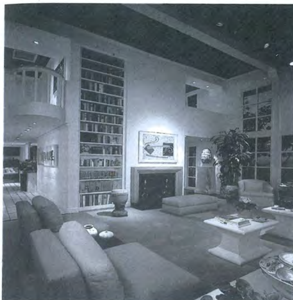
Figure 18-24. This living room features a 25-ft wooden ceiling to which 4-circuit track is mounted on both sides of the beam. All the track heads are positioned at less than a 25-degree aiming angle. The lighting contributes to the feeling of calm, spaciousness, and relaxation.
