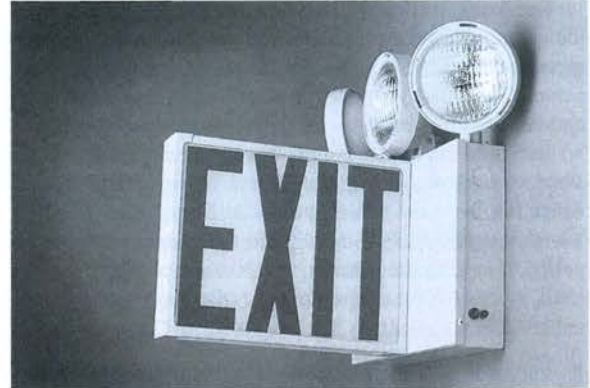
Figure 29-6. Directional emergency lighting equipment can create disability glare and compromise the efficiency of evacuation. In smoke, luminaires can reduce the visibility of exit signs along the same line of sight.
