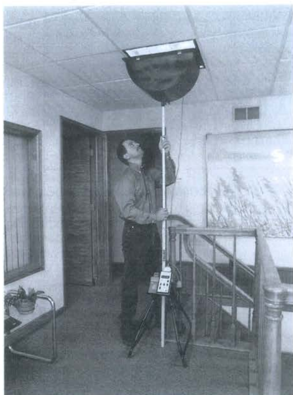
Figure 28-2. A fluxometer developed to measure a luminaire's available light in order to determine the benefits of periodic cleaning.
