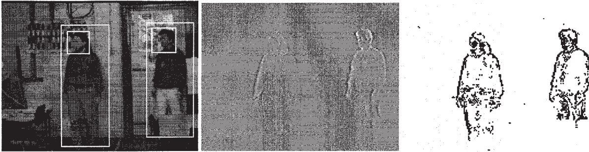
Figure 1. The motion-based tracker. Left: An image from a sequence taken in our lab with bounding boxes for the tracked people and their heads overlaid. Centre: The image after temporal convolution. Right: Detected temporal zero-crossings.
