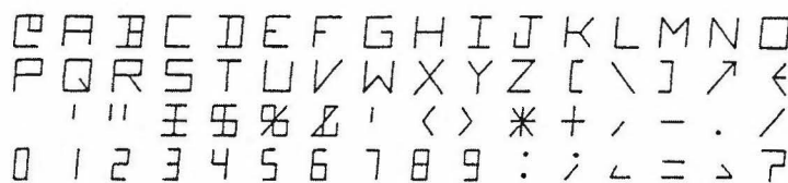
FIGURE 35.8 (a) LED display formats; and (b) displayed alphanumeric characters using 16-segment displays.
