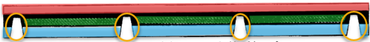
G. Notch process along the dice lines, carried from the back side of the wafer.
