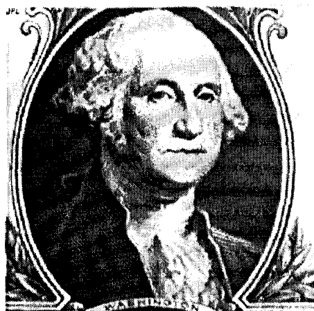
Figure 8. Image of a US $1 bill taken with a JPL 256x256 element CMOS APS showing excellent image quality with no artifacts.
