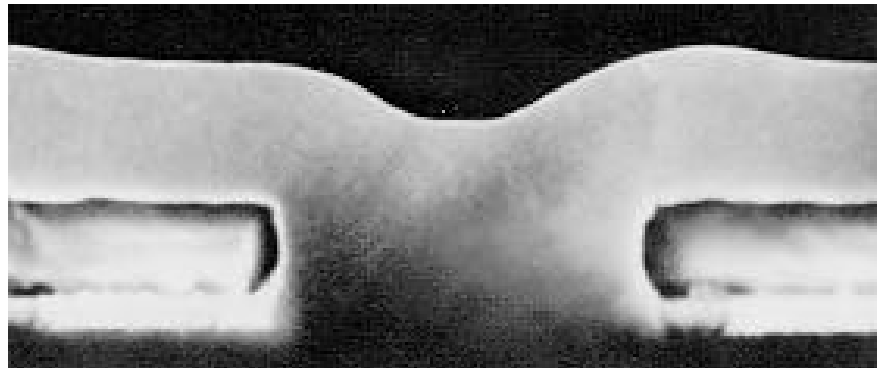
1 \mu\text{m} planarization etchback
