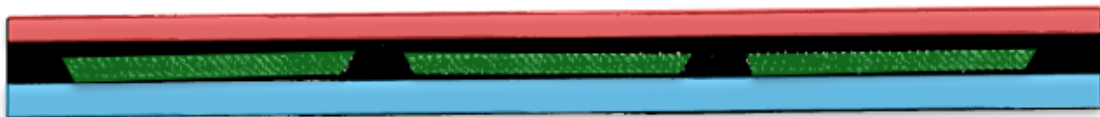
F. Attach a second glass plate from the back side, the epoxy fills the trenches between the dies.
