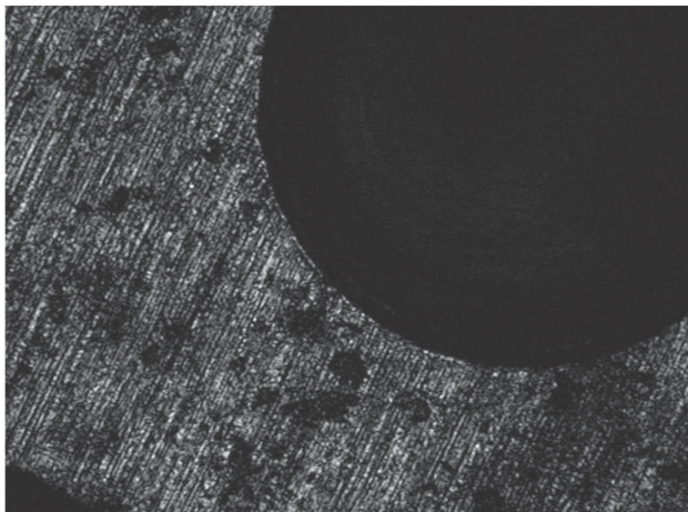
Fig. 2. Optically sectioned images, taken at focal settings 1.25 mm apart, of a section of a wrist watch mechanism: the scale bar depicts a length of 100 \mu\text{m} .
