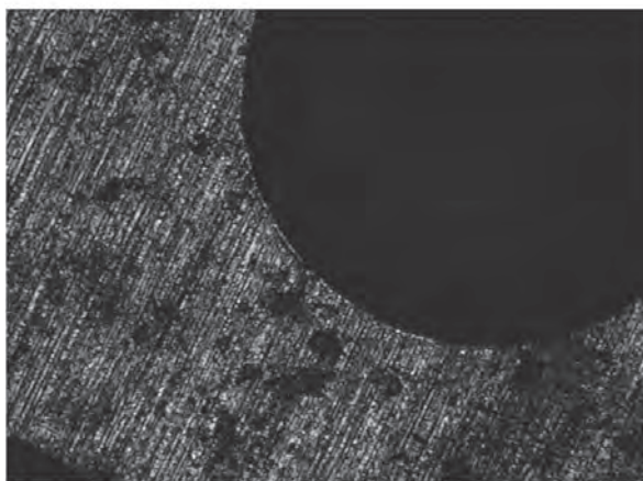
Fig. 2. Optically sectioned images, taken at focal settings 1.25 mm apart, of a section of a wrist watch mechanism: the scale bar depicts a length of 100 μm.
