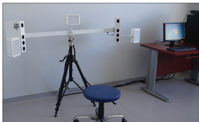
Figure 4: Stereophotogrammetry with 2 different coplanar planes for 3D images
