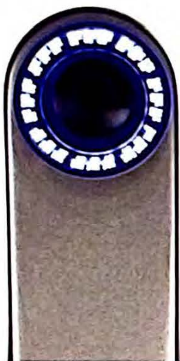
Figure 15 The tip of the wand contains 192 LEDs and 22 lens systems and captures impression and occlusal registration data in video mode.
