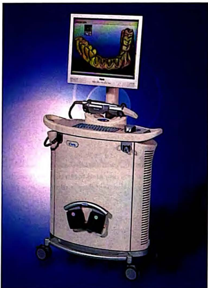
Figure 9 The iTero 3D digital impression system. Scan data of preparations are e-mailed wirelessly to Cadent for creation of the model, which then is sent to the laboratory for the restoration.
