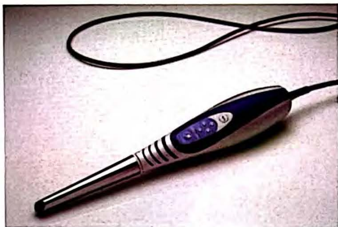
Figure 14 The Lava C.O.S. camera has the smallest wand of any of the reviewed systems, making access to all parts of the oral cavity easier to achieve.
