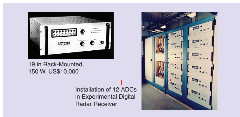
FIGURE 9: The HS-810, an 8-bit, 10-Ms/s ADC released by Computer Labs in 1966.
