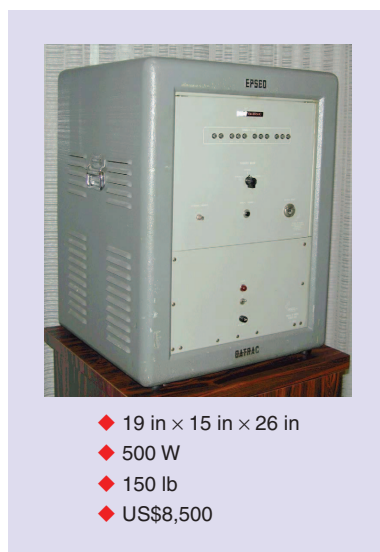
FIGURE 8: 1954 Epsco Datrac 11-bit, 50-kSPS vacuum tube ADC designed by Bernard M. Gordon of EPSCO. (Reproduced with the permission of Analogic Corporation, Peabody, Massachusetts.)
