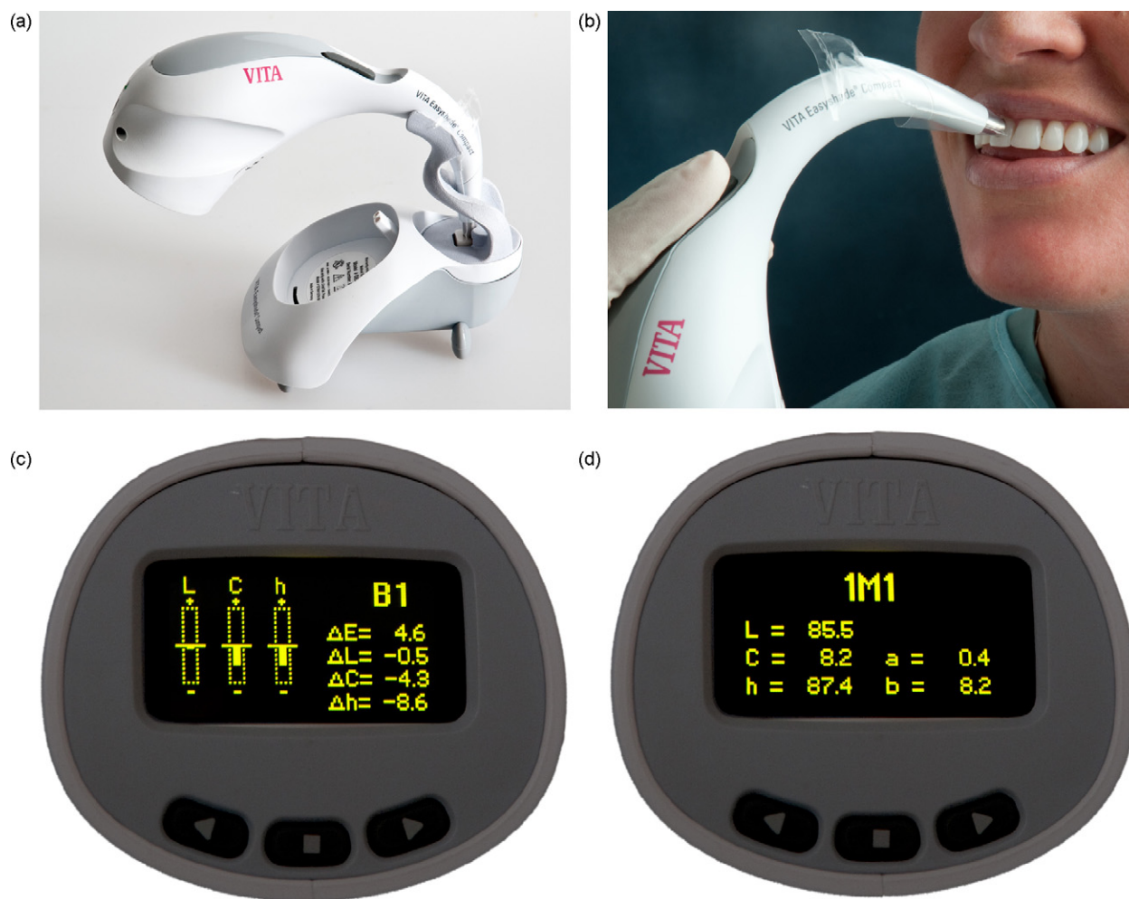
Fig. 2 – Clinical application of EasyShade Compact spectrophotometer. (a) Instrument calibration. (b) Color measurement. (c) Color difference metric values as compared to the corresponding Vitapan Classical shade. (d) Color coordinate values and the corresponding Vitapan 3D-Master shade.
