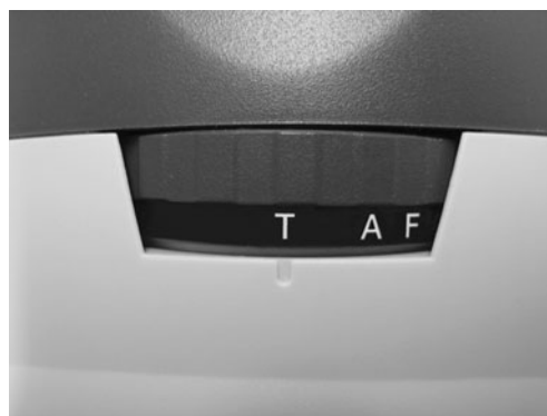
Fig. 3 Level of the depth of focus can be switched between tooth (T), lips (A), and facial (F) position. For the purposes of this investigation, the level of focus was selected on position T
