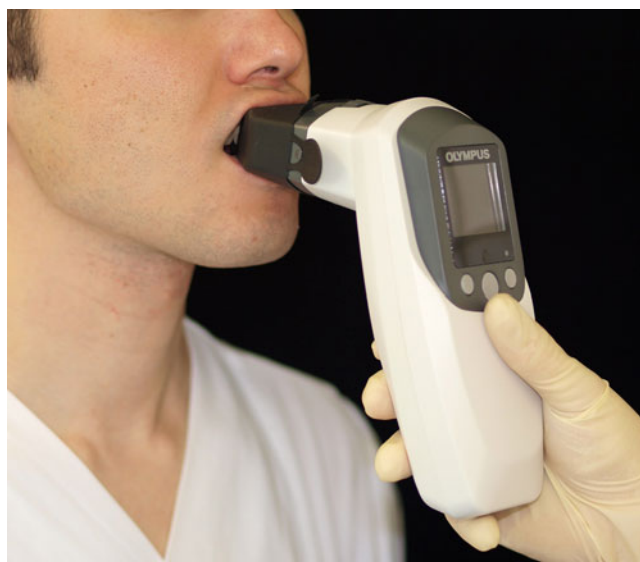
Fig. 2 Data acquisition with the digital spectrophotometer used in the study. The measurement was performed with a single-use cap for each patient
