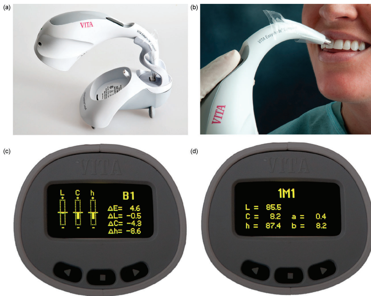
Fig. 2 – Clinical application of EasyShade Compact spectrophotometer. (a) Instrument calibration. (b) Color measurement. (c) Color difference metric values as compared to the corresponding Vitapan Classical shade. (d) Color coordinate values and the corresponding Vitapan 3D-Master shade.
