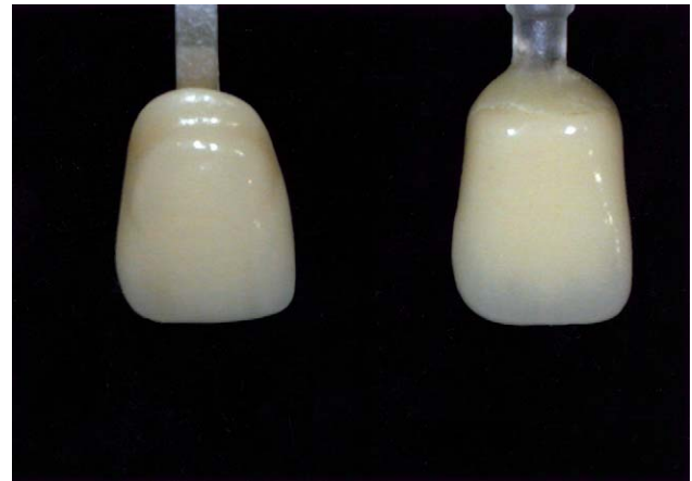
Fig. 5. Target-shade tab 3M-2 and corresponding CCM ceramic specimens. (Left: Target-shade tab 3M-2, Right: CCM specimen)
