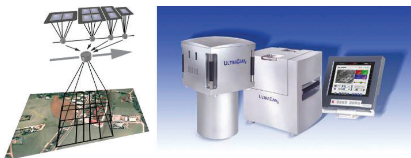
FIG. 11. (a) Concept of the Microsoft UltraCam large-format digital camera—showing the arrangement of the four lenses mounted along the flight direction and the multiple CCD area arrays that are used to generate the final panchromatic image. (b) The principal components of the Microsoft UltraCam-X model with (from left to right) the camera unit with its recessed handles; data storage unit; and user display screen ( source : Microsoft).
