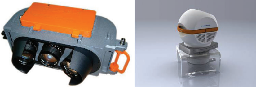
FIG. 17. (a) The 3-DAS-1 three-line pushbroom scanner produced jointly by Wehrli & Associates and Geosystems features three Kodak trilinear arrays, each with a separate lens, to produce continuous colour linescan imagery (source: Wehrli & Associates). (b) The Jena-Optronik JAS 150 three-line pushbroom scanner (source: Jena-Optronik).
