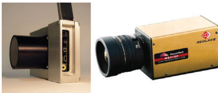
FIG. 5. (a) Tetracam ADC Air camera. This is an inexpensive small-format camera designed specifically for use in airborne agricultural and environmental monitoring based on a 3.2 megapixel CMOS area array. Once again, the colour images are produced using a mosaic filter and Bayer interpolation ( source : Tetracam). (b) Redlake MS4100 camera. This is based on the use of three CCD area arrays, each with a 1\text{k} \times 1.9\text{k} pixel format, and a beamsplitter placed between the lens and the three arrays. Each array has its own spectral filter ( source : Redlake).
