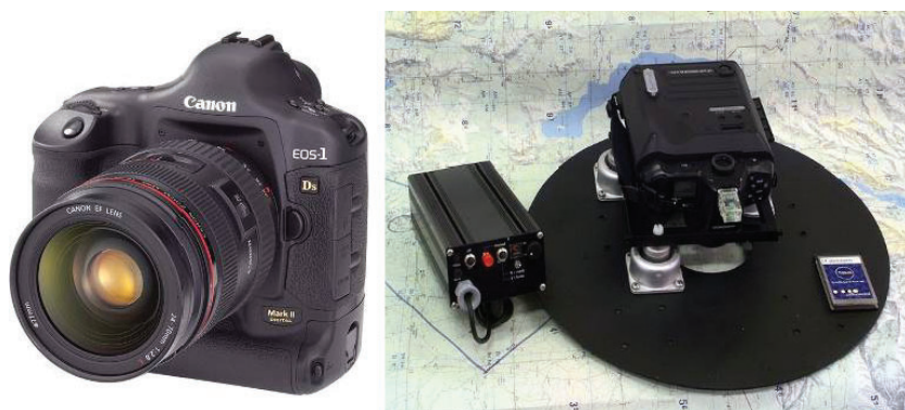
FIG. 4. (a) The Canon EOS-1Ds Mk. II camera, based on a CMOS area array, acquires images with 16.7 megapixels. This camera produces its colour images using a mosaic filter and Bayer interpolation ( source : Canon). (b) GeoTechnologies' SF-DMC small-format digital camera with an anti-vibration mount based on shock absorbers and an electronic control box ( source : GeoTechnologies).
