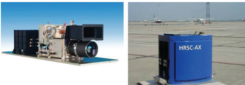
FIG. 15. (a) The DLR HRSC three-line stereo pushbroom scanner was developed originally for the Russian Mars96 mission. It is now being used on the ESA Mars Express mission. (b) The HRSC-AX (Airborne Extended) version of the HRSC scanner is equipped with a narrow-angle lens and an integrated GPS/IMU unit (source: DLR).
