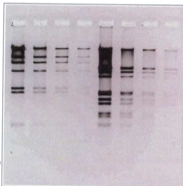
Fig.5-2 Detection of SYBR® Green-stained \lambda DNA / Hind III Left : SYBR® Green excitation / Blue-LED emission spectra Right : Example of detected image
