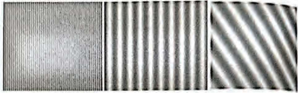
FIGURE 1.11 Sinusoidal objects. Spatial frequency examples: high frequency, mid frequency, and low frequency at a different azimuth angle.
