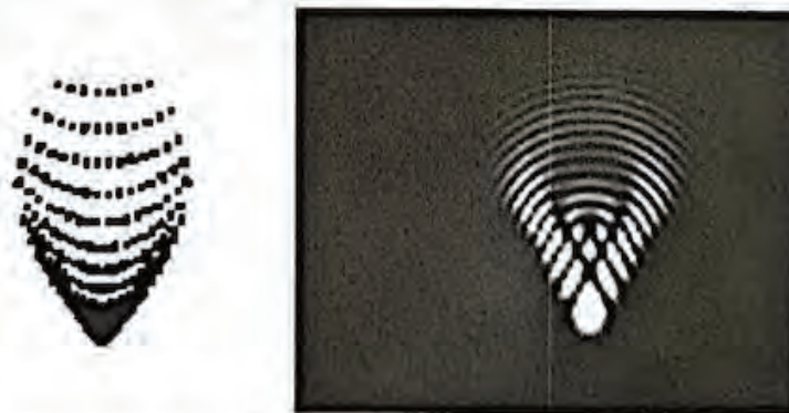
FIGURE 1.9 Example of a geometrical PSF of an aberrated star image from a grid of traced rays ( left ), and a similar PSF including the wave nature of light ( right ). The shape and size of the images compare, but the details differ significantly.
