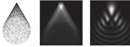
Figure 9.6 Spot diagrams for five waves of coma aberration. Left, standard spot; center, binning and counting rays; right, diffraction calculated.
